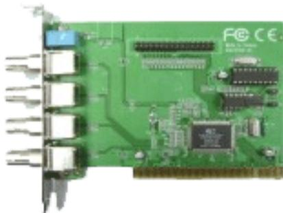
**Capture Card-** Connects inside Computer and analog camera connects to it.
