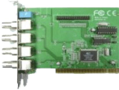
If you are using a capture card, not every capture card will work. Most capture cards are designed to work only with the software that came with the card.
